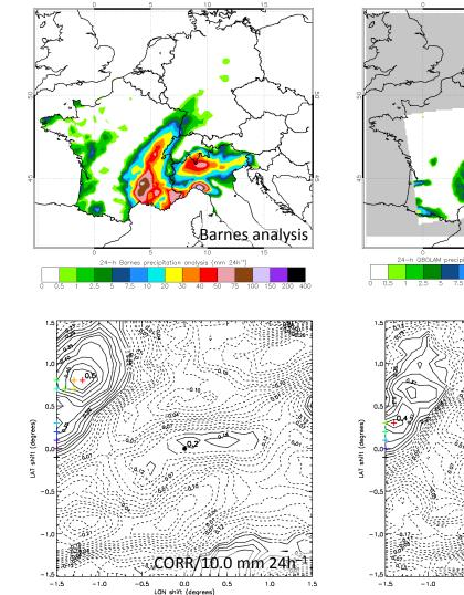
PHASE BOLAM 24-h QBUAM precipitation field on a 0.1" regular grid (mm 24")
